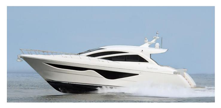
DRAGON 72- DEA DEL MARE is one modern high speed express yacht with European style and stream-line shape based on the customization to owner's preference. The yacht is with 22 meters in length, 5.3 meters in width, and maximum speed up to 34 knots and the hull structure is designed on the DNV high speed light craft code and complies with Japanese JG regulation.
