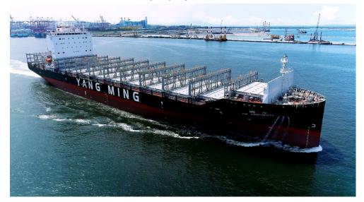
"YM Continuity" is one of the series container ships, which are designed, built and delivered by CSBC. This ship, with lower fuel consumption features, will further reduce the owner's operating costs, comparing to older, or chartered-in vessels. This vessel is applied with energy saving technologies, including twisted rudder, asymmetry rudder bulb, high efficiency propeller, CSBC unique SSB (Sea Sword Bow) and smart-ship technologies.
